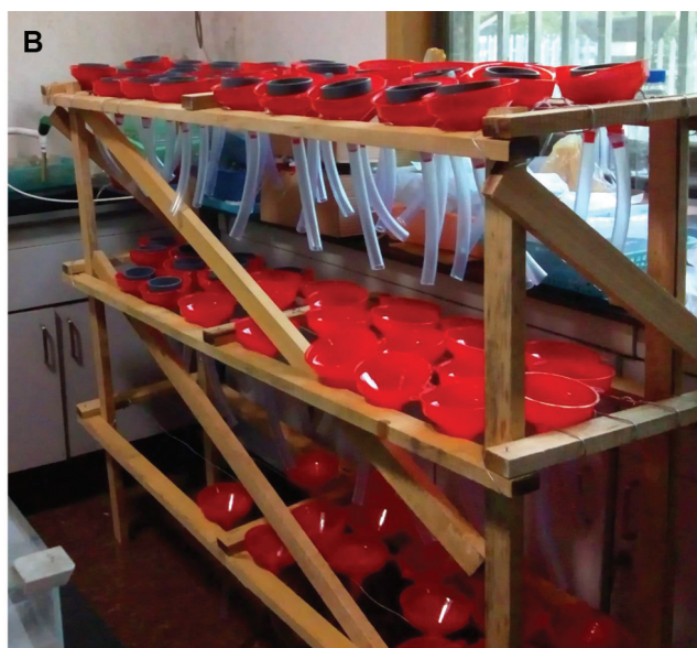
Figure 1. (A) Schematic Baermann-funnel apparatus for nematode extraction from soil. (B) Wooden frame to carry single Baermann funnels build in China with simple materials (Photo credit: Rémy Beugnon).
